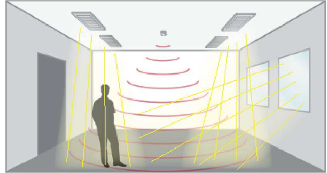
Presence detected some daylight. Lights are ON and dimmed to maintain lux level
